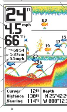
**Cursor Dialog Box** - indicates cursor depth on the display In addition, the Latitude and Longitude of the cursor position and the bearing to the cursor position. A waypoint
